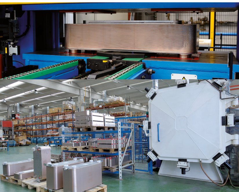
In the fully automatic test machine the brazed plates heat exchangers are tested for a working pressure up to 30 bar (45 bar for the H version).
