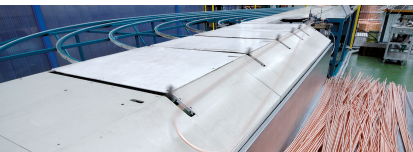
A fully automatic machine cuts, bends and works the evaporators copper tubes, which are internally rifled.
